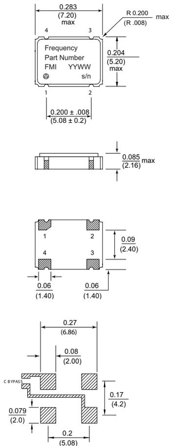
An external bypass capacitor 0.01μF is required between Vcc and GND
