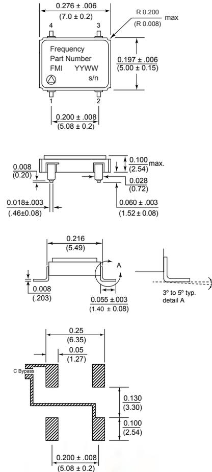
An external bypass capacitor 0.01μF is required between Vcc and GND
