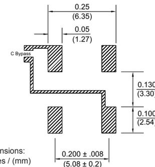
Leads are integral to the ceramic header. They are **not** added on to the package in a post manufacturing process.
