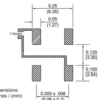
Leads are integral to the ceramic header. They are **not** added on to the package in a post manufacturing process.
